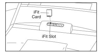
Next, select an iFit workout by pressing the iFit increase and decrease buttons next to the iFit slot. When an iFit workout is selected, the display will show the duration of the workout, the maximum incline setting, the workout number, and the maximum speed setting of the workout. In addition, a profile of the speed settings of the workout will scroll across the matrix.
